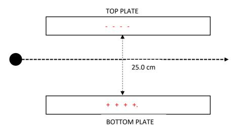
(a) Use the data above to calculate the potential difference (V) between the two plates.
